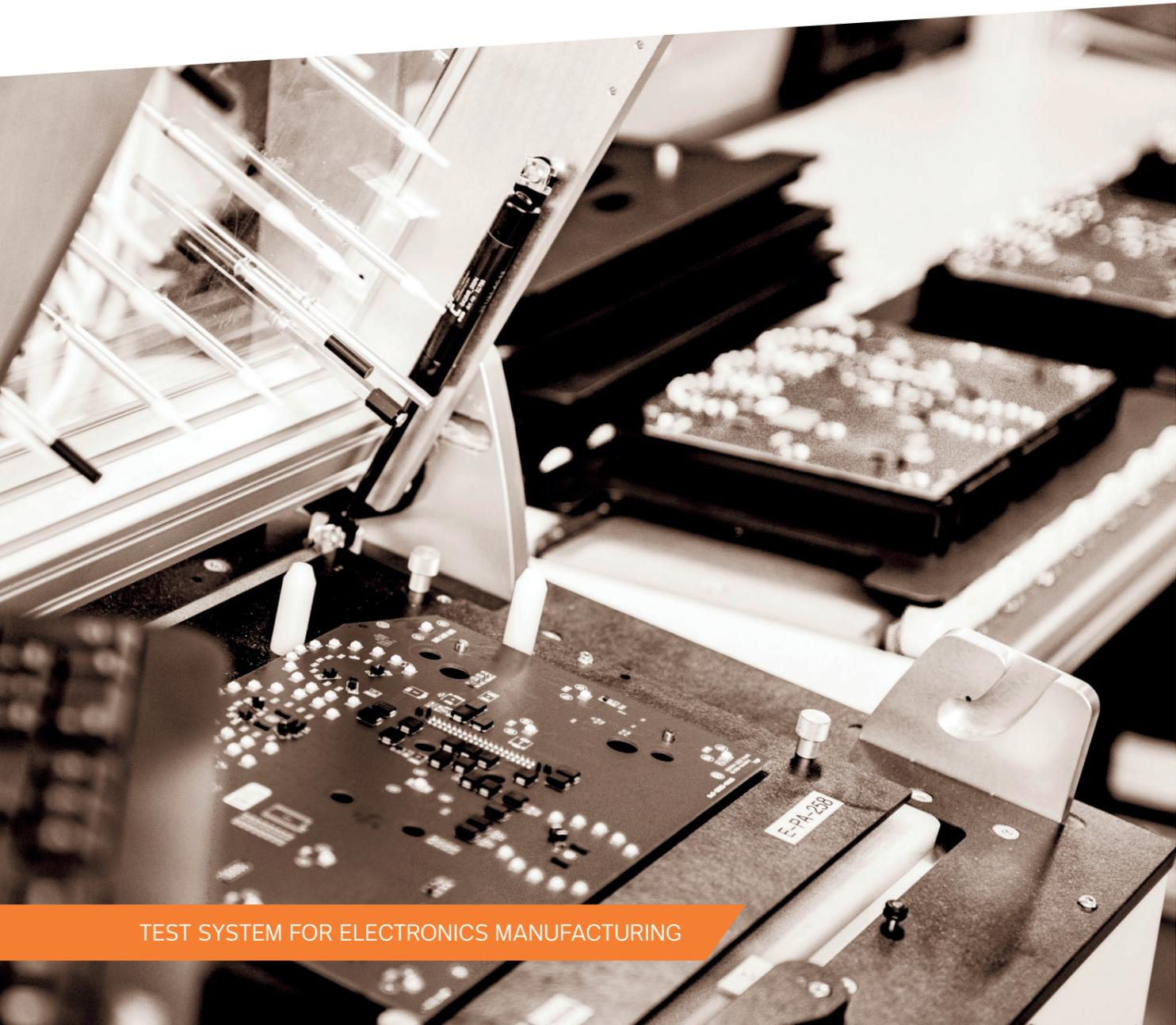
TEST SYSTEM FOR ELECTRONICS MANUFACTURING
